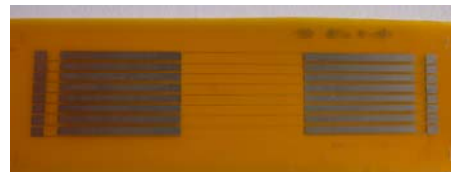
Figure 9: New HFS with thin film technology (wire thickness 30\mu\text{m} ) [28]
